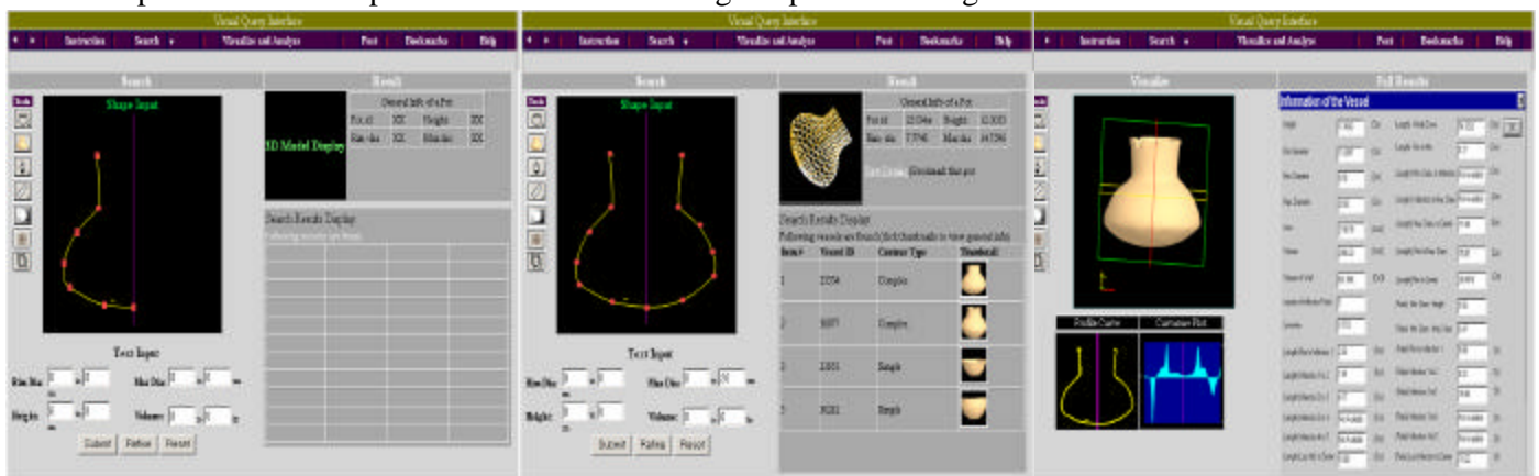
Figure 6. (L to R) Query interface screen with sketch-based, numeric, and text-based input fields. Initial response screen with resulting thumbnail images and summary data, and wire frame of first matching vessel. Detail individual display screen with 2D, 3D, and descriptive vessel data.
